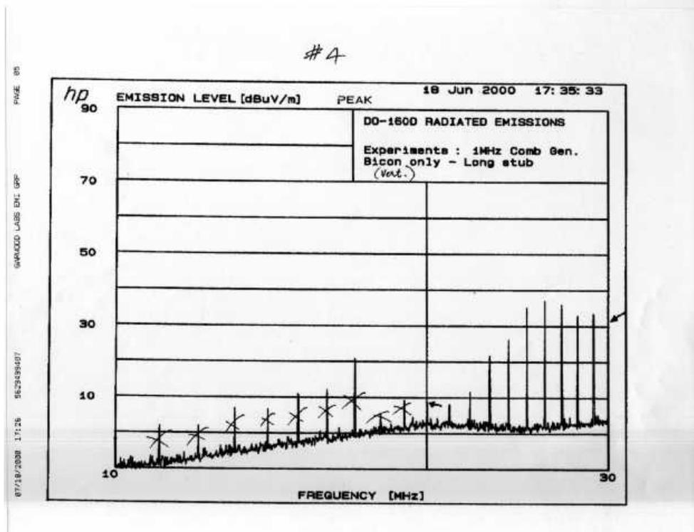
Figure 7 – Vertical Biconical Antenna Measurements \*
