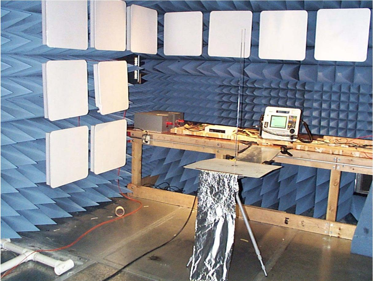
Figure 3 – CKC Rod antenna setup and experiment
